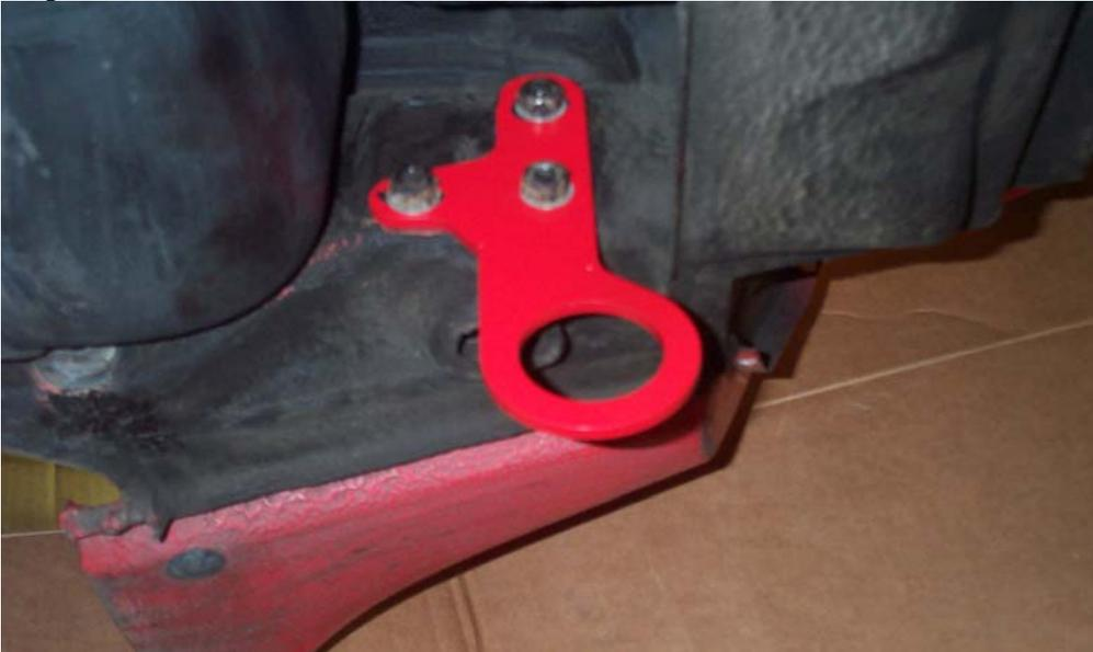
Remove nuts. Install bracket as shown. Note: You may want to apply some sealer around the studs to prevent water leaking into the trunk. Install and tighten nuts.
