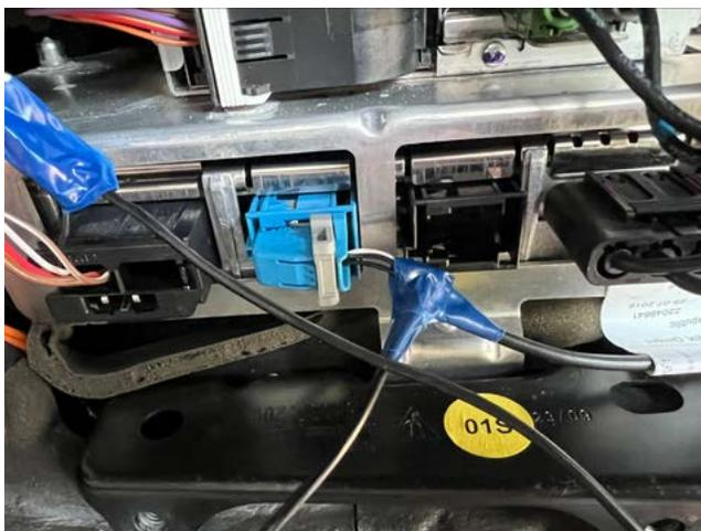
**Please note** that the OEM TV module is only FO bypassed, it must be still connected to the power cable.
