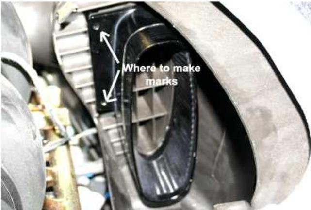
7. Using a marking tool, make 2 marks on the OEM air box where the billet filter collar bolt holes will attach to the OEM air box.
