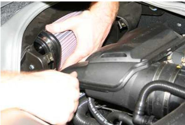
13. Slide filter into OEM air box housing and attach the filter to the billet filter collar. Make sure the filter is as far on the collar as possible.
