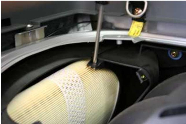
4. Remove the 1, Phillips head screw that attaches the OEM filter to the air box.
