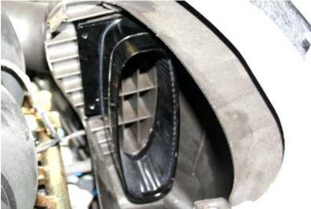
6. Attach the black V-Flow billet filter collar to the OEM air box by snapping it into the OEM filter port inside of the air box. Make sure that this collar is fully in place before moving on to the next step.
