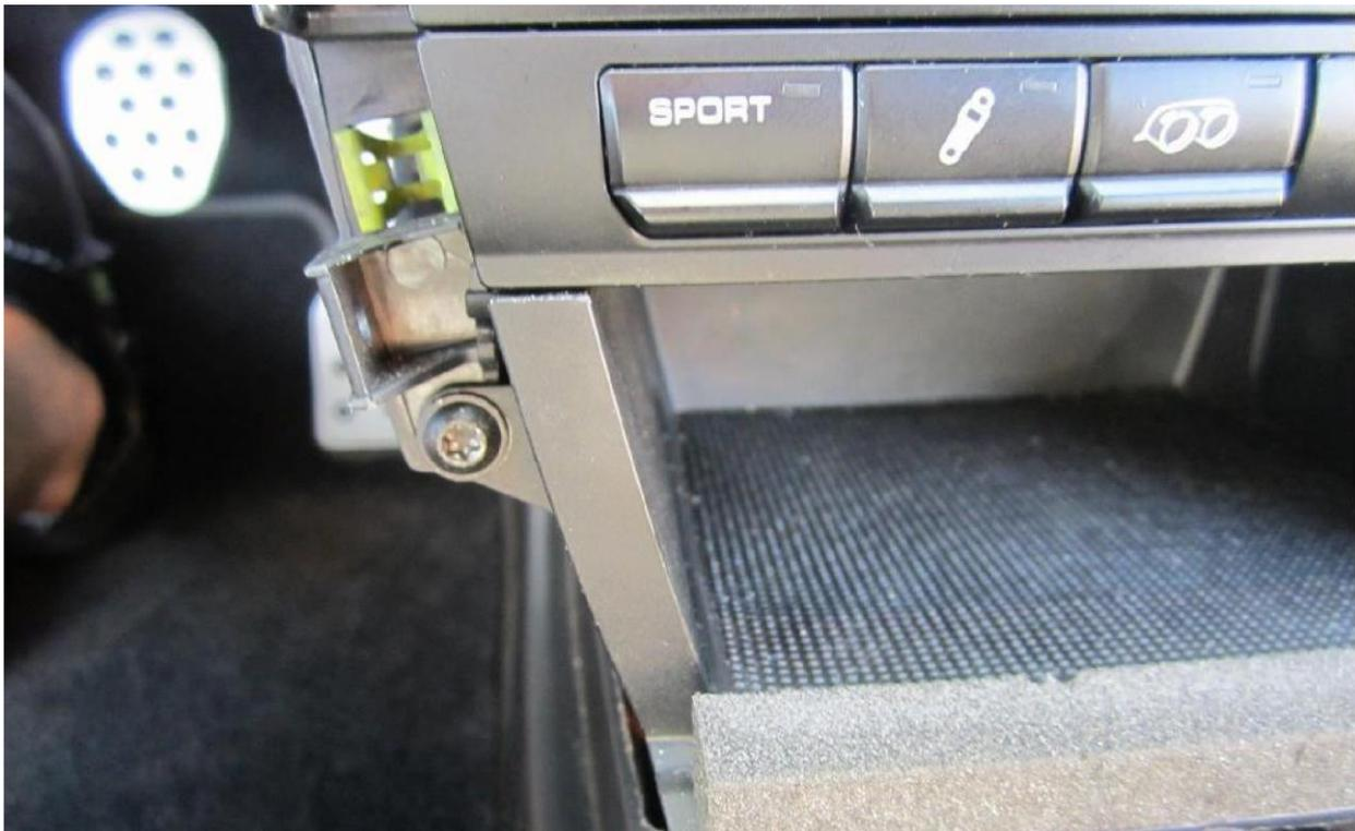
8. You are ready to pull the console out but first locate the wire connector on the inside right front of the console and disconnect it. Have the emergency brake handle pulled up. Pull the console up and out of position.
