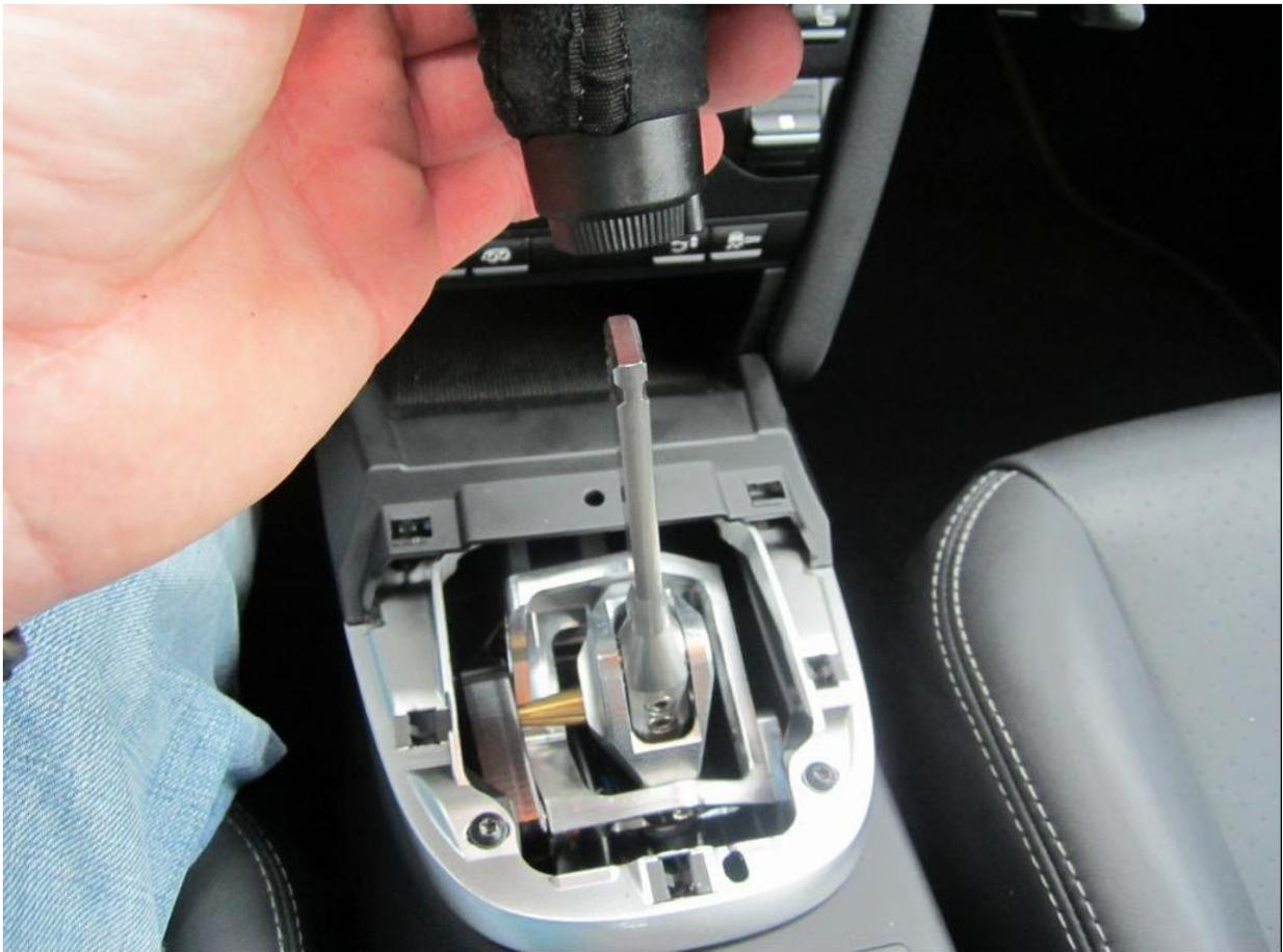
5. Remove the 4 torx screws holding the shifter trim on. You will have to pop 2 snap clips out to get to 2 of the screws. Then pull the trim off.
