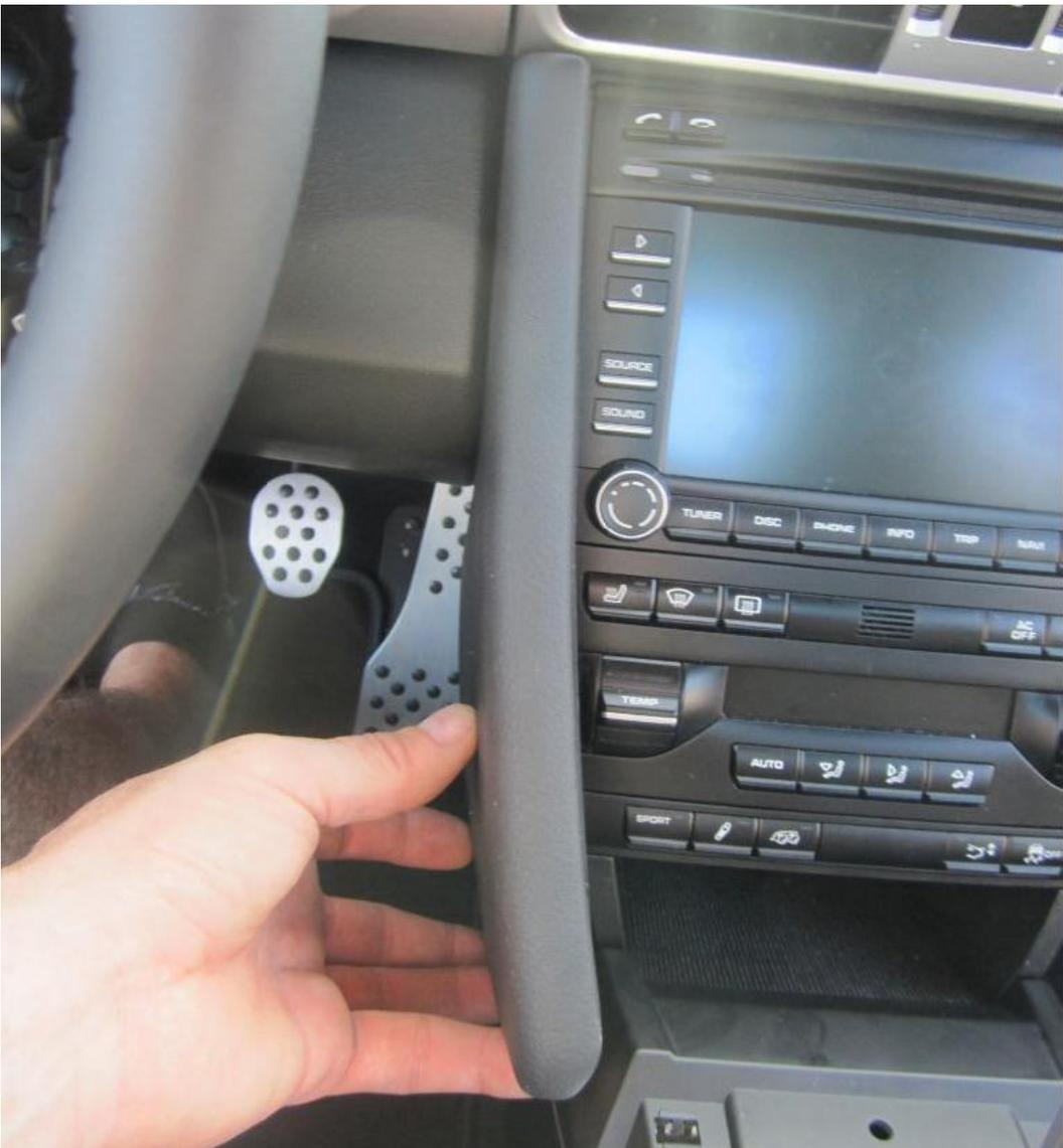
7. Remove the 2 T20 torx screws holding the very front of the console on. Next remove the 2 T20 torx screws holding the the storage tray on just below the radio. Pull the storage tray out by pulling it straight out. Last remove the one T20 torx screw under the storage tray holding the console in.
