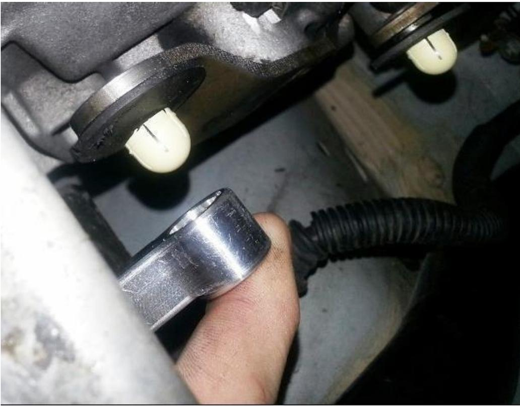
The ball bearing rod end is fully adjustable and attaches to the left side of the shifter (not tightened).
