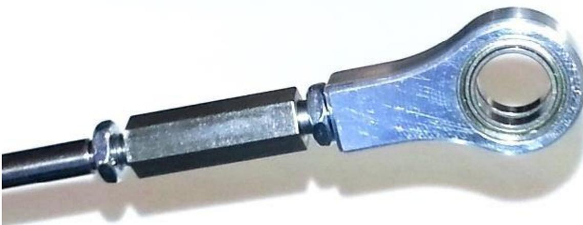
Adjustment will move shift lever position. Be sure to have it's in the desired position before securing.
